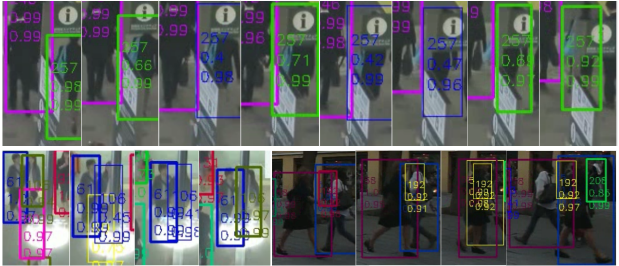
Fig. 3. Qualitative examples of our framework. Thick colored : identified tracklets associated with a detection. Thin blue : non-associated tracks being kept active because of their confidence score. Thin yellow : inactive tracks. In each box, the first number is the target identity, the second is the detection confidence score and the third is the tracklet reidentification score with the associated detection or predicted position. The first row and left half of the second one illustrate cases where keeping a confident track active pays off under scene occlusions. The right half of second row shows a type of identity switch our framework still struggles with. For better viewing, a video is provided as supplementary material.
